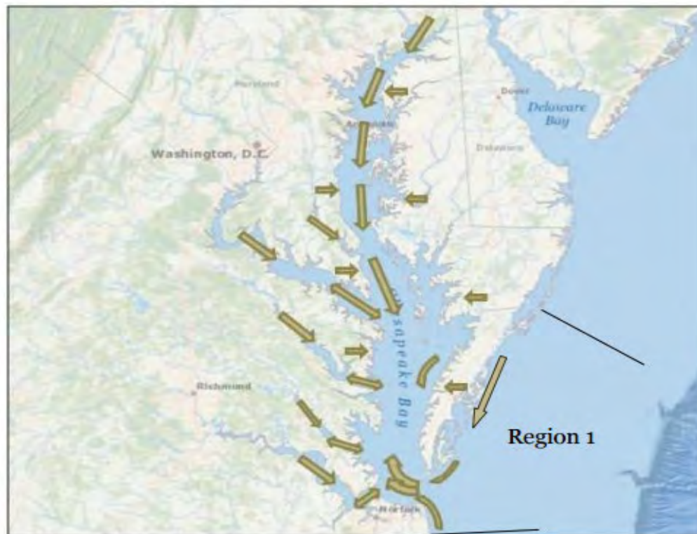
Figure 2: Net sediment transport pathways for Chesapeake Bay and Atlantic area off the Virginia Coast. Source: "North Atlantic Coast Comprehensive Study Report (USACE, 2015).
